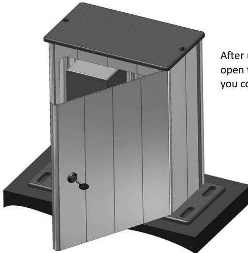
After unlocking with the enclosed key, you can open the door up to an angle of 140°. This gives you convenient access to the inside of the drive.
